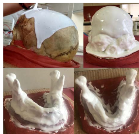
Figure 3: Silicone pouring layer by layer on the skull and mandible
